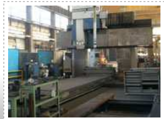
CNC portal milling Waldrich FP 180 x-y-z:8000x1800x1400mm
